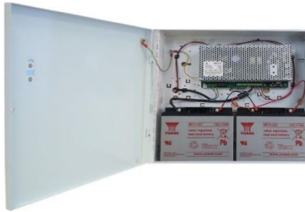
Figure 4 – Battery backup supply
