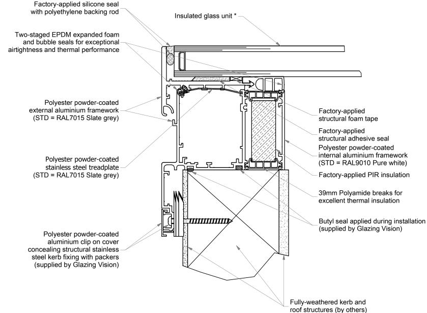
\*Standard double glazed unit comprises: 6mm Clear HST toughened outer 20mm Warm edge argon filled silicone sealed spacer 6mm Clear HST toughened soft coat low E inner
